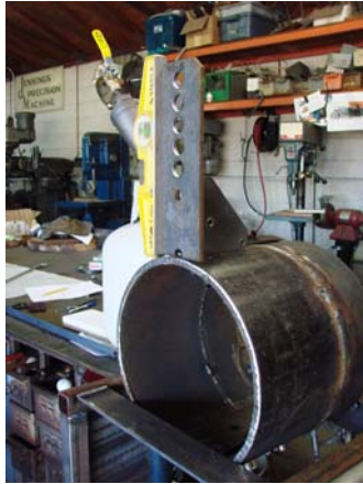
It takes some trial and error to decide on the height of the holes that will work with your doors. Hold it with a magnet, plumb it with a level, weld in the gussets. Weld in the hooks that hold the door on after installing the Kaorwool.
