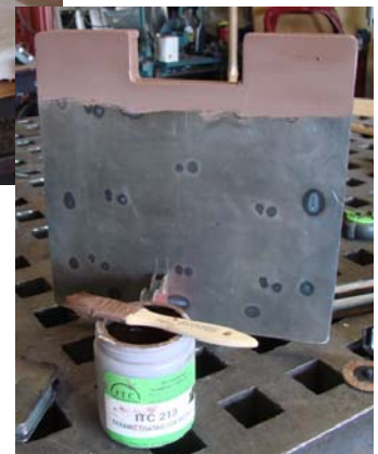
The bottoms of the doors see a lot of heat as the flame exits through the notch and under the door. I coat the bottom angle and about 3" up on the door skin with ITC 213, which is a ceramic coating for metal. I then paint the door with high temp (2000 deg) header or BBQ paint. Using stainless steel for the bottom angle and notch (or even the entire door) would provide another measure of durability, but may not be worth the extra cost.
