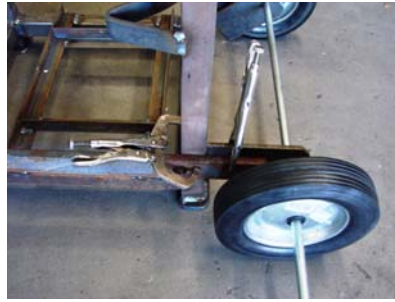
Wheels and stand are on the floor. 1/4 x 3 plates with a hole locate the wheels. A straight bar and clamps line them up. Below: With the wheel brackets welded in and the axle cut to length, hammer on the push nuts. A little mass on the opposite end makes the installation easier.
