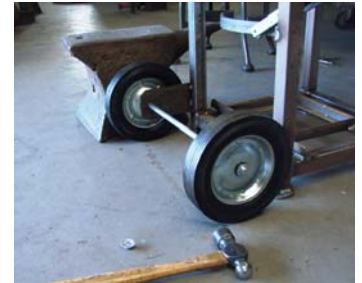
Wheels and stand are on the floor. 1/4 x 3 plates with a hole locate the wheels. A straight bar and clamps line them up. Below: With the wheel brackets welded in and the axle cut to length, hammer on the push nuts. A little mass on the opposite end makes the installation easier.
