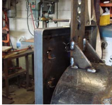
It takes some trial and error to decide on the height of the holes that will work with your doors. Hold it with a magnet, plumb it with a level, weld in the gussets. Weld in the hooks that hold the door on after installing the Kaorwool.
