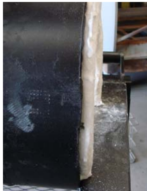
I use a carpenter's square and a utility knife to cut the Kaorwool. The Kaorwool should stick out of the housing about 1/4" on each side and butt against the side of the brick. Cut a hole so the Kaorwool fits tightly around the burner.
