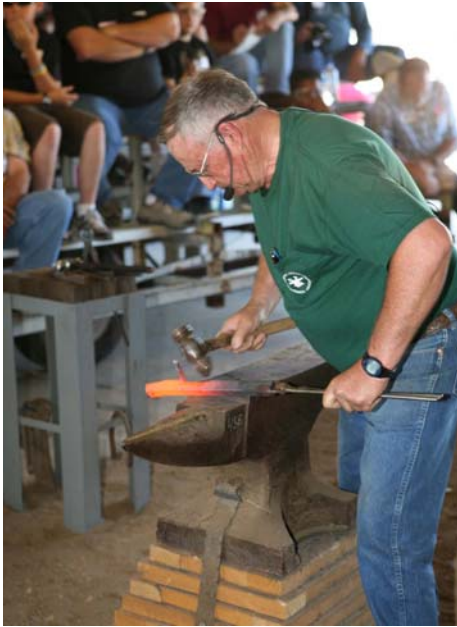
L: Demonstrator Jim Keith working on his Dragon head. He started with 1" square stock and drew out the neck to create a handle for the shovel.
