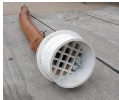
Photo 4 & 5: Exhaust adaptor/connector with leather air tube. Opposing views
