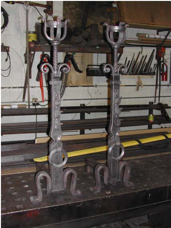
Andirons, 46" tall. Forged from 1 1/2 x 3 Steel
