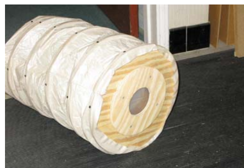
Photo 2. Bellows air bag made from a shower curtain and plywood ribs.
