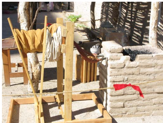
Photo 1. Proof-of-concept bellows and adobe forge ready for a living history demonstration at the Presidio San Augustin del Tucson in Tucson, Arizona.
