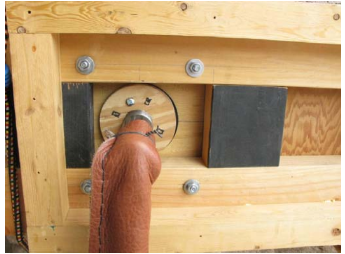
Photo 6: Exhaust adaptor/connector with leather air tube fitted into the end of one of the air bags which is mounted, with four 3/8 x 16 bolts, on the vertical frame.
