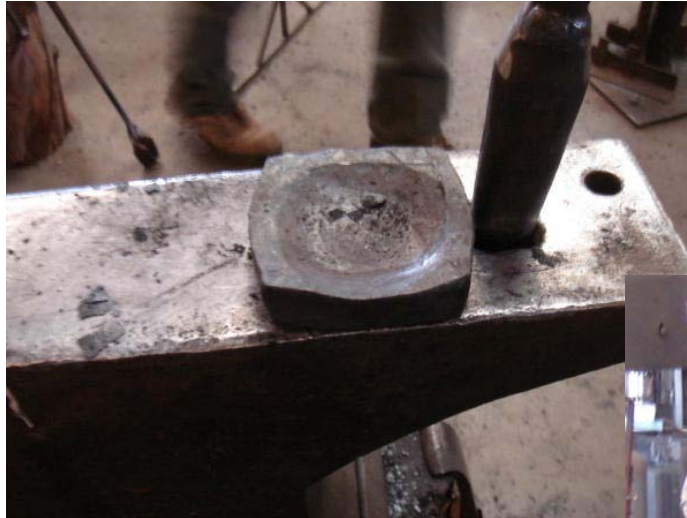
Left: die used to shape the round end of the rounding hammer and the eye drift
