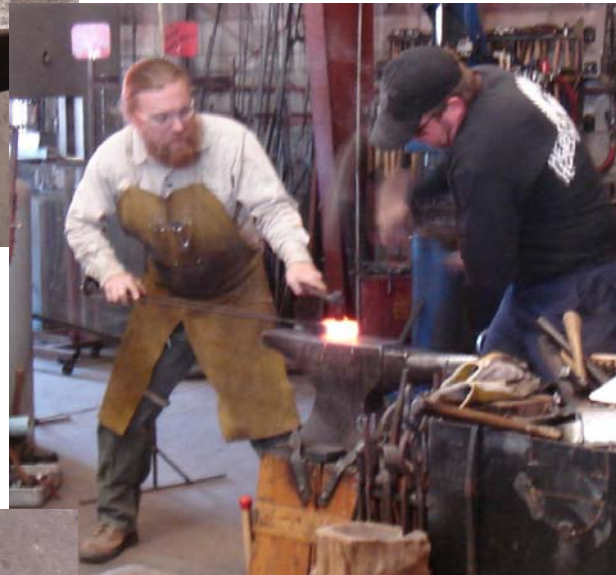
Below: James McLaughlin strikes for Pep. They are punching the slot for the hammer eye.
