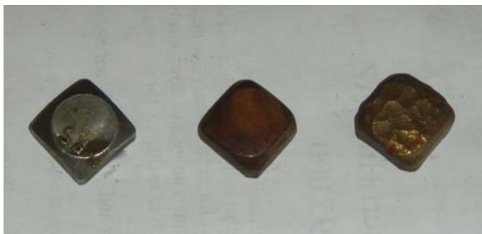
Photo – Left: start with this, Middle: smooth finish with muriatic acid/hydrogen peroxide patina, Right: bumpy texture with Japan Brown patina).
