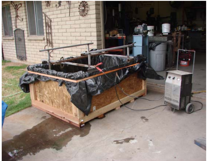
Etching tank. I had Lowes cut the sheets on their panel saw (they don't charge for the cuts). The heavy plastic had a couple small holes . This required that I leave the hose trickling with just the right flow so that it didn't over fill and reach the charger clamp or go too slow and leave the part uncovered. I also added washing soda every few hours. It was a mess.
