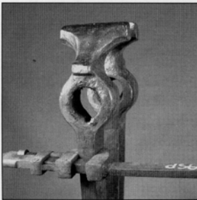
Fig 8. Correcting for racked jaws; the joint was clamped in another vise for protection
