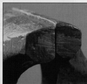
Fig 2. Jaws do not align vertically
