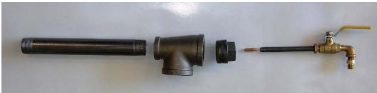
Burner parts: (Left to Right) 1” x 10” black pipe nipple, 1 1/2 x 1 x 1 1/2 black pipe tee, 1 1/2 black cored plug, .045 MIG tip, 1/8 x 1/2 schedule 80 pipe nipple, 1/4 x 1/8 MIP x FIP brass bushing, 1/4 full port threaded ball valve, 1/4 brass 90 degree street elbow, 1/4 MIP x left hand gas fitting. Note: The MIG tip should have 1/4-28 threads. Get that size nut and take it to the welding supply, they will have no idea what you are asking for. While you’re there get the 1/4 MIP gas fitting. Source: PEXSupply.com has most of the fittings, Grainger 1/8 sched 80 nipple (pn ILLV2), Airgas MIG tip and left hand gas fitting.
