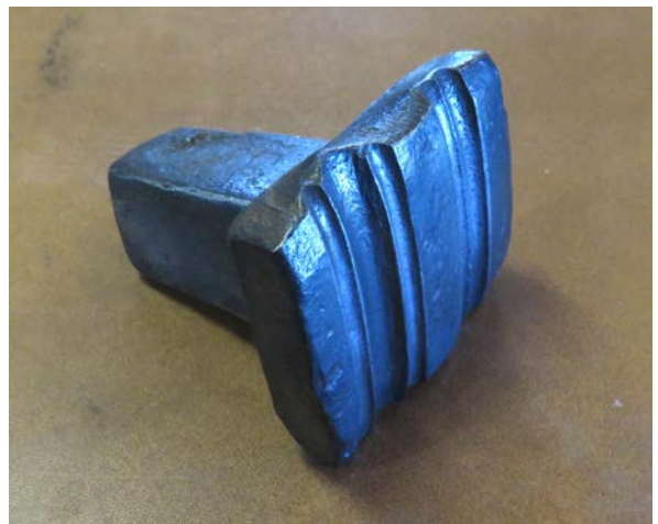
The swage block (hardy) for texturing the collars. This block had ridges for both the large and the small collars.
