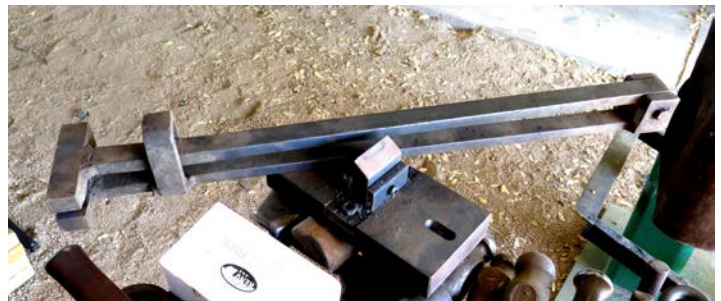
Detail of the wavy tail (left) and the die (above and below left) that John used in his treadle hammer to shape the tail.
