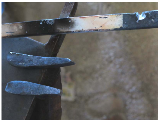
Results. The water cooled bit is on the bottom.
