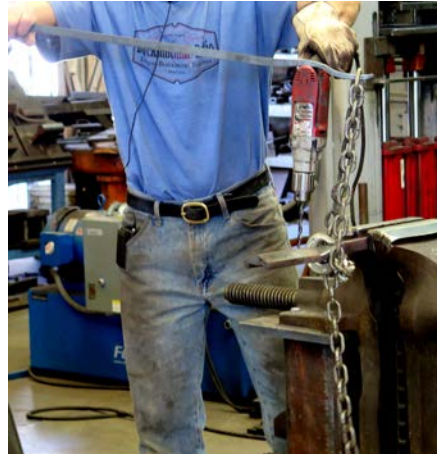
Lever for applying extra pressure for drilling
