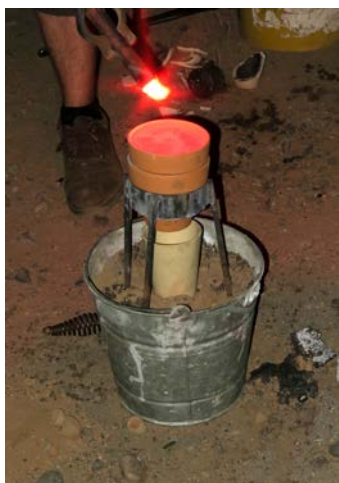
Load the thermite into nested flower pots, light it with a road flare, and let the molten iron and slag drop into a high-temperature crucible.
