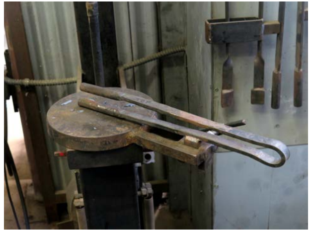
Fuller on the treadle hammer
