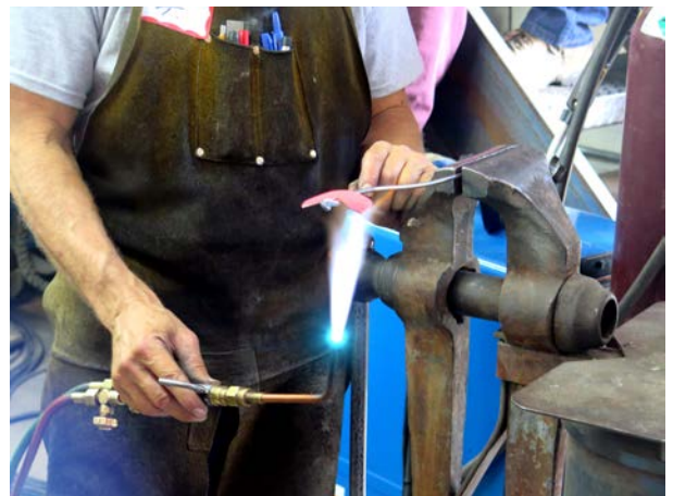
Fusing the enameling powder to the work piece
