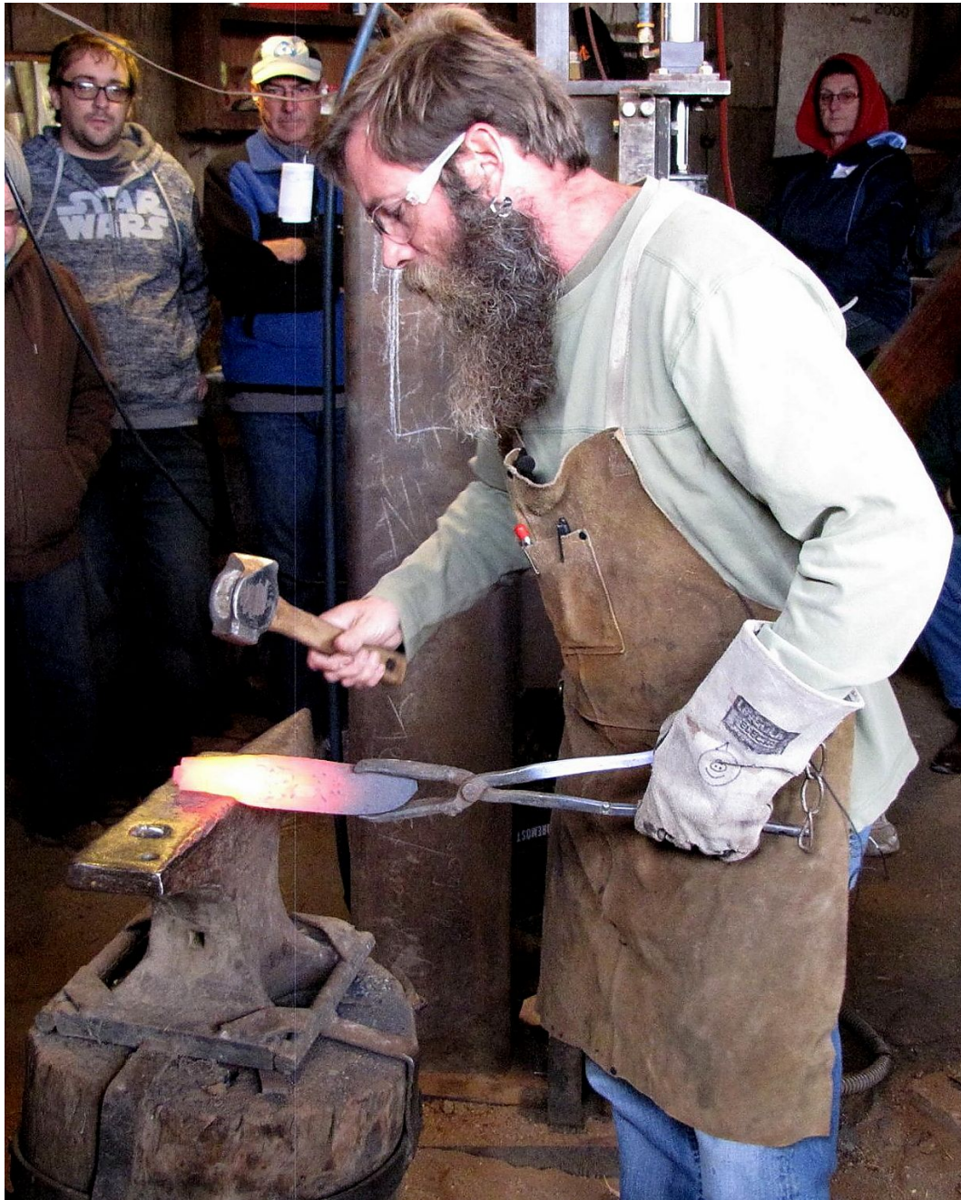
Rich Greenwood forging a san mai knife at the AABA demonstration in Tucson, January 21, 2017
