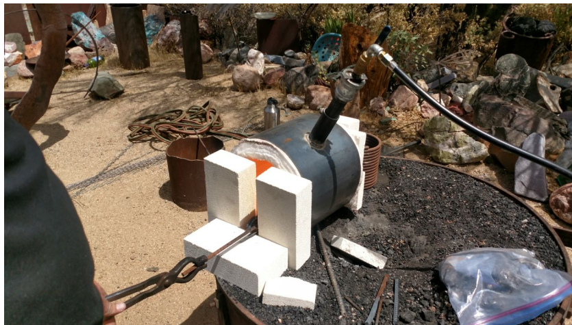
One of the propane forges built at Dief's forge building workshop last April.
