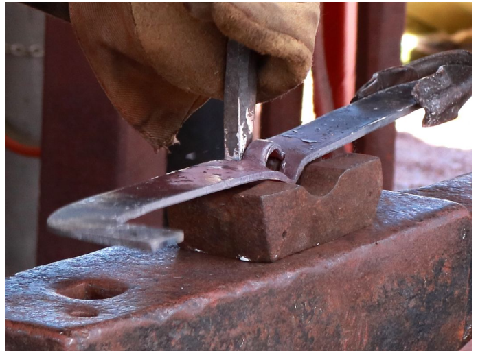
Forming the slotted pass-through joint
