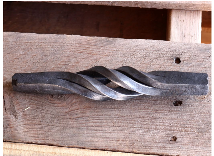
Jay's basket twist created by forge welding four rods together.
