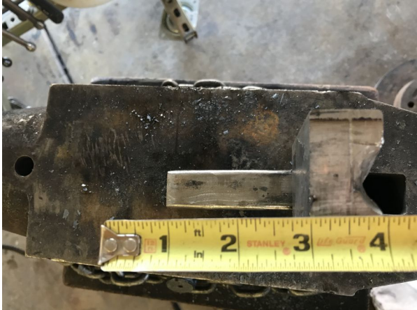
Hardy tool with dimensions
