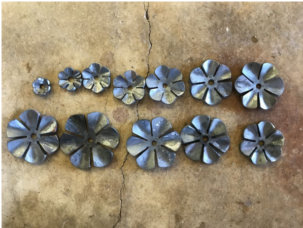
The 12-segment pine cone kit after shaping each segment
