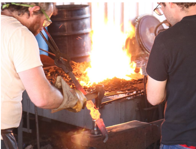
Haley Woodward (l.) necking down a work piece.
