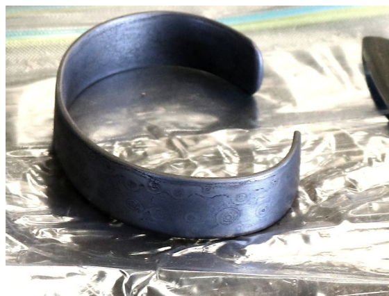
Show and Tell - by Moe Hamburger 40 layers of old butter knives (sheet steel) and one layer of wrought iron - forge welded in an induction forge.
