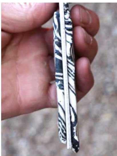
San mai: hard steel for a good edge sandwiched between two pieces of pattern welded steel.
