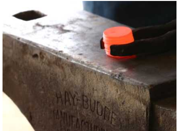
A successfully welded coin stack ready to for flattening and developing the visual pattern.
