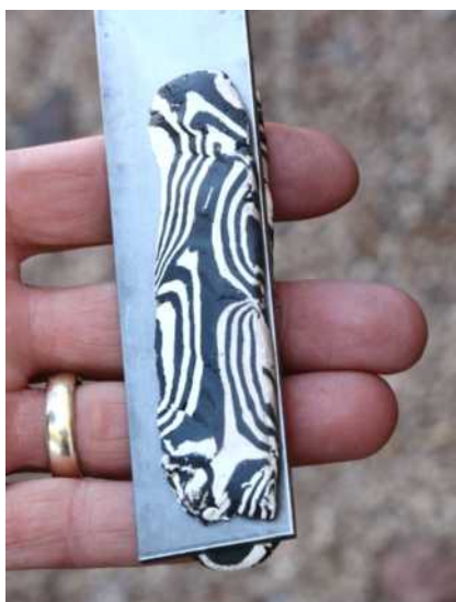
San mai: hard steel for a good edge sandwiched between two pieces of pattern welded steel.
