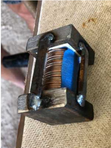
A stack of quarters held in a welded cage in preparation for forge welding the coins.
