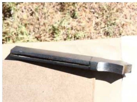
The start of a one-piece spur. Brian allowed as how he cut the slot with a band saw.
