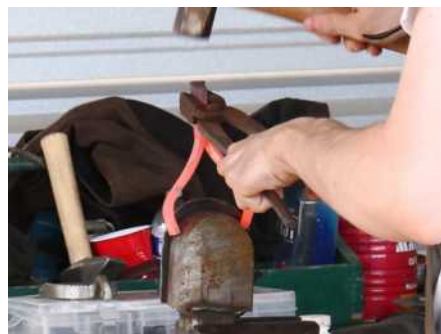
Shaping the band on the one-piece spur using Brian's shop-made form.
