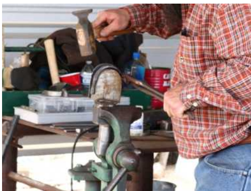
Brian used one of his shop-made forms for final shaping of a band for a two-piece spur.
