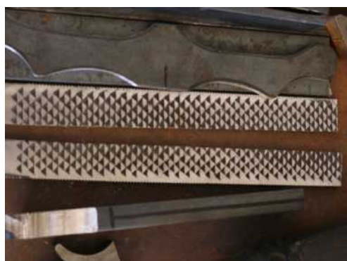
A couple of farrier's rasps with teeth flattened to be used as straps for a pair of spurs.
