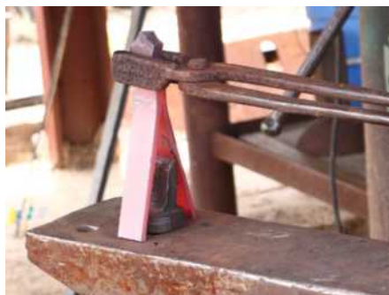
Opening the slot to make the band for a one-piece spur
