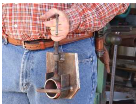
Brian demonstrated one of his jigs for bending a strap for a two-piece spur.
