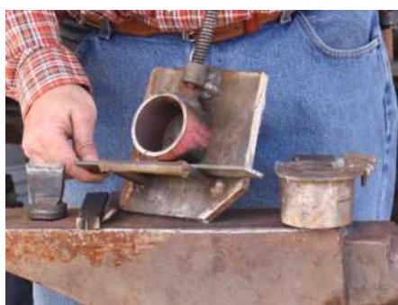
Brian demonstrated one of his jigs for bending a strap for a two-piece spur.
