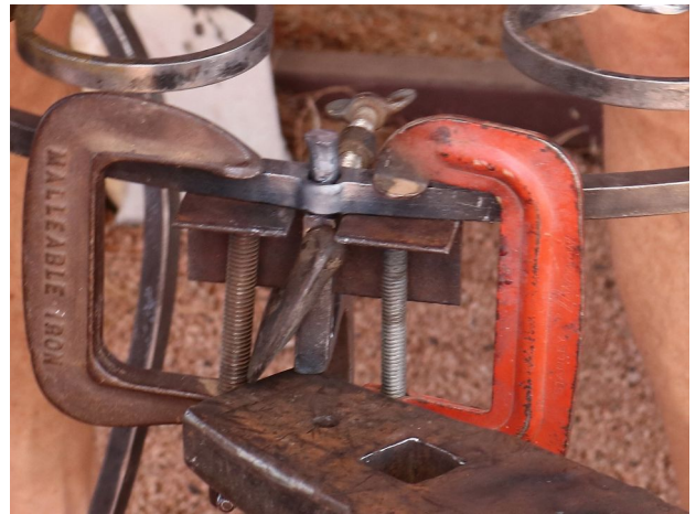
Set up for heading the leg tenon. Note how the shape of the legs allows for using the anvil face when upsetting the tenon head.
