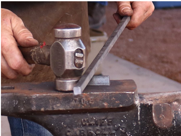
Nicking the square rod with an anvil devil
