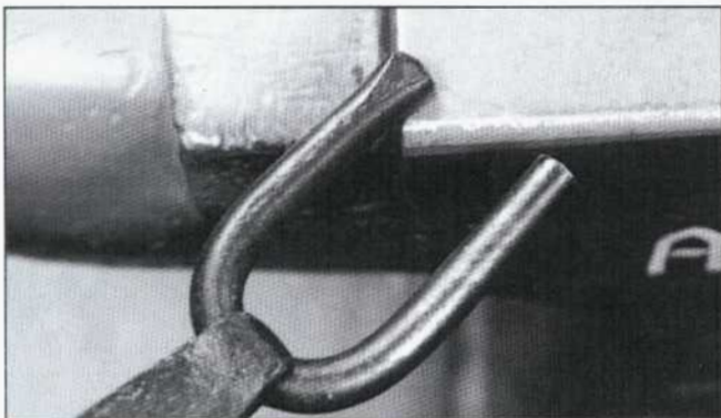
Pivot around the bottom contact point
