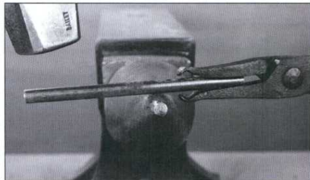
Bend the bar either at the bick or in the pritchel hole
