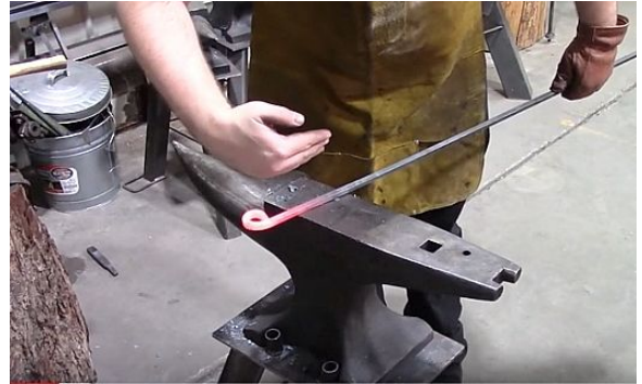
Matt explained making consistent tripod leg.
