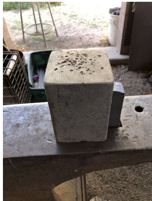
Trex punch block with hardy stub
