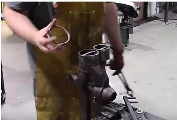
Matt showed how he used the jig he made to help make the rings.
