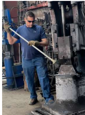
An important job for Kurt's assistant was to sweep away the scale while the work piece was in the forge.
