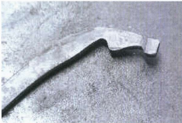
Above: Bend the nose down a little and pull out the mane with the cross peen.
