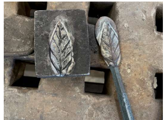
A leaf die and a leaf made with the die.
