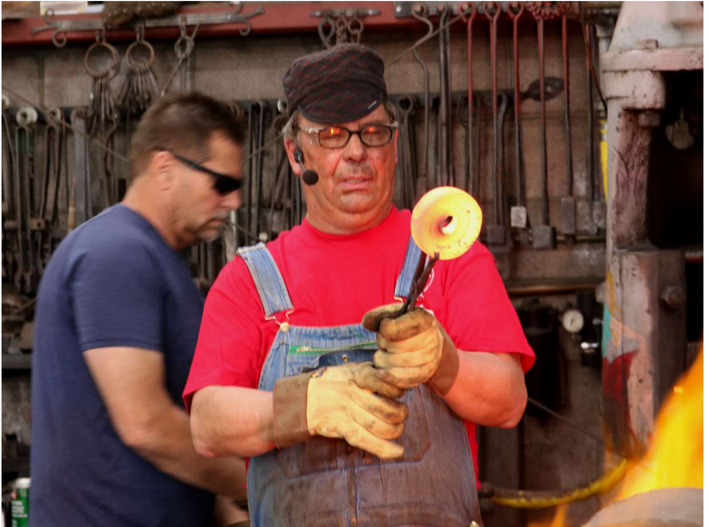
Our March demonstrator, Kurt Fehrenbach, making a bushing.
