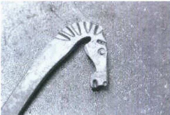
Below: Ear, mouth, eye, nostril, and the mane. That's actually three heats: Ear and mouth, then eye punch and nostril, and then the five marks for the mane.
