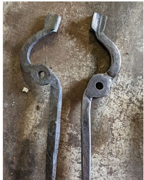
Making the tongs - ready for the rivet
