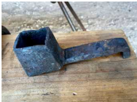
Partially finished baluster stiffener by Jacques Gallant which he used as an example for his demonstration on Friday morning.
