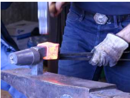
Jacques Gallant creating a truncated square taper from a short piece of round tube using a purpose-build hardy tool.
