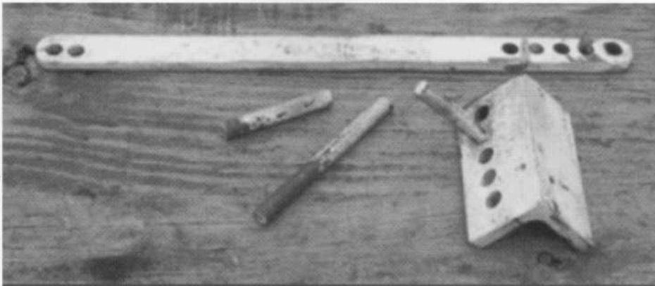
Bender parts, handle, base, three pins
