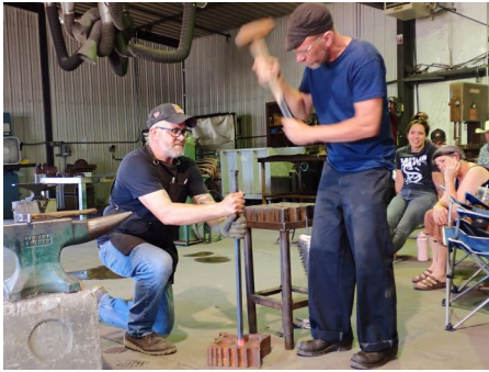
Dylan Cook (l.) and Mike Riemer upsetting the round end of a leg using a swage block.
