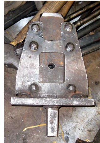
Dylan's guillotine with dies for making the tenons. (photo by Terry Porter)
