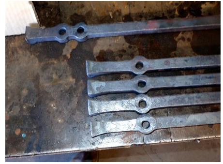
Legs punched, upset, and ready for assembly.
