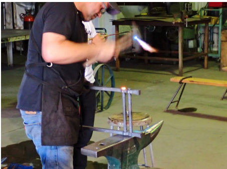
Dylan Cook creating a rivet head on one of the tenons.
