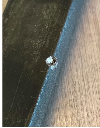
Marked with a center punch at the edge of the bar
