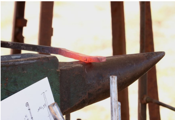
Drawing out over the horn of the anvil.
