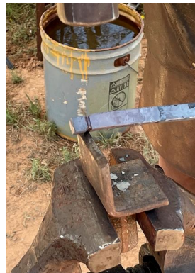
Starting a tenon with a sharp butcher (made from angle stock).
