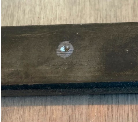
Marked with a center punch in the center of the bar.
