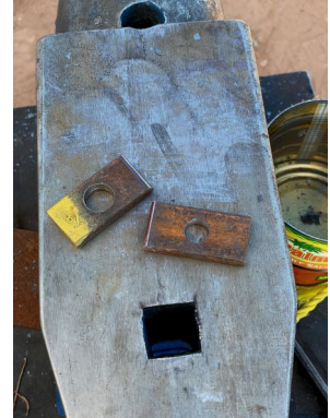
Small bolsters sized for punching a particular project
