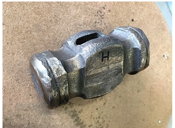
The finished rounding hammer.
