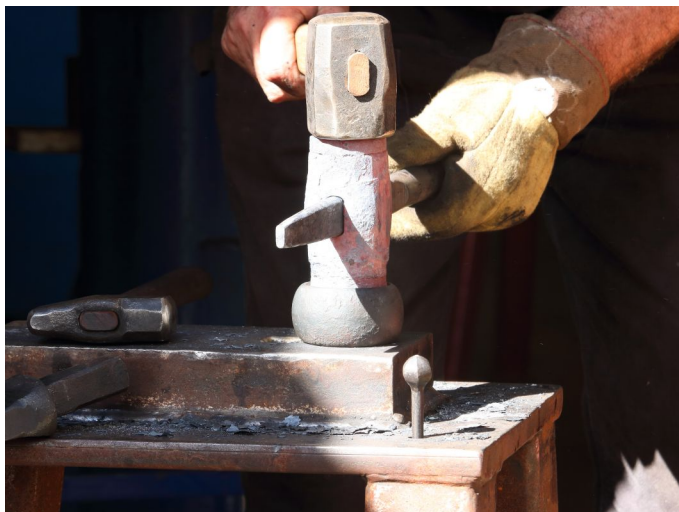
Final forming of the hammer faces. The rounding face is being formed in a shallow bowl .
