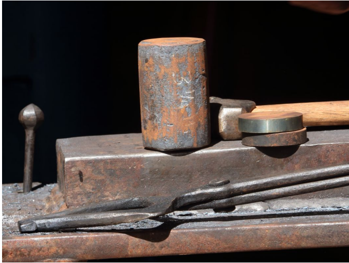
The start of the wrought iron hammer with the tool steel faces
