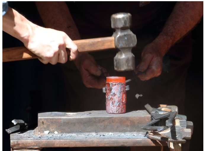
Welding one of the tool steel faces onto the wrought iron body.
