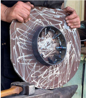
The jig Dylan had made for forming the large loop of the scroll.
