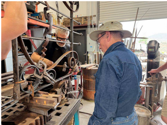
Fitting the scrolls into the gate in preparation to drill the rivet holes. (photo by Mikki Rakestrow)
