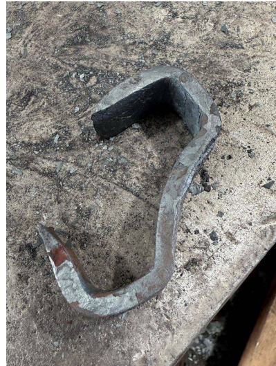
The same collar opened up and ready to be installed on the gate.
