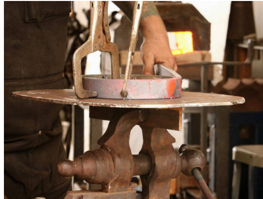
Wrapping a bar around the jig. Vise-grips are your friends.
