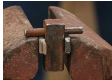
Filing rectangular tenons for final fit.
