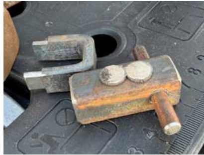
Using rare-earth magnets to hold collars in place while shaping them.
