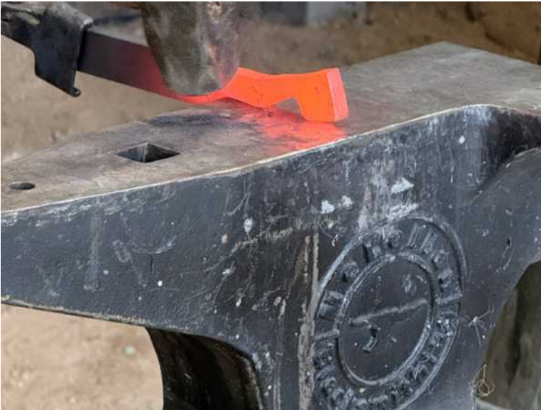
Setting the shoulders for tongs based on Dylan's design.
