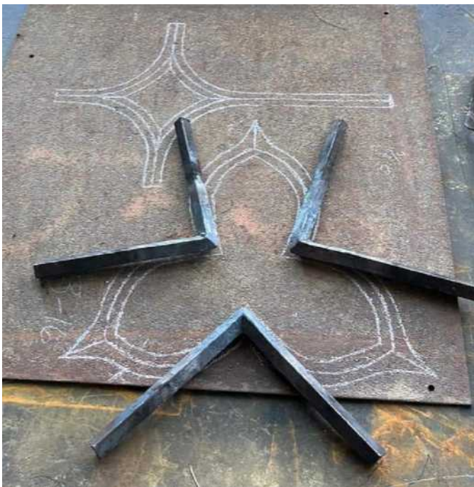
Below: Three right angles on the layout table before bending.
