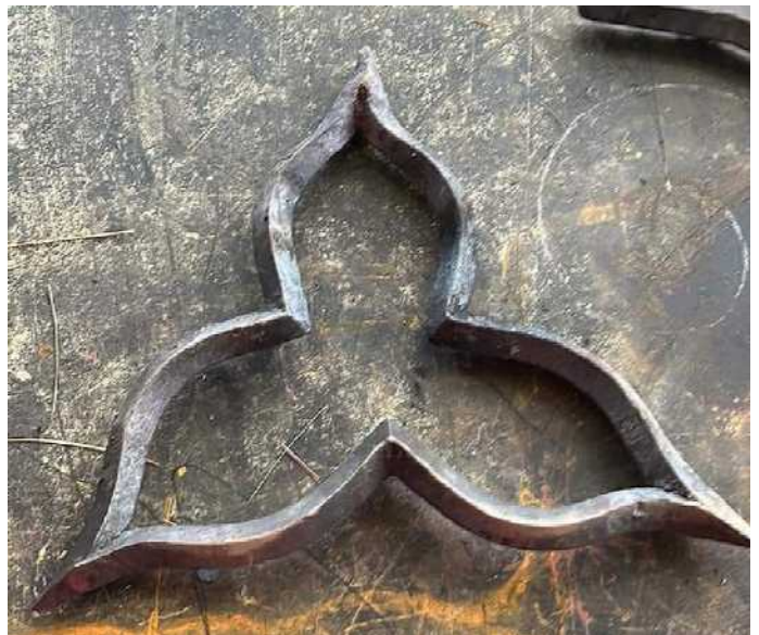
Below: The trefoil with the corners welded and forged to clean points with facets and corners neatly centered.
